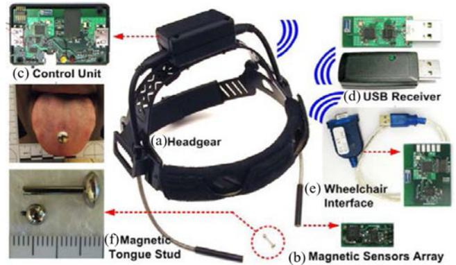
Fig. 1. (a) eTDS prototype used in this study consists of a headgear (b) with an array of three-axial magnetic sensors (c) mounted on a pair of goosenecks and a wireless control unit. (d) Wireless receiver USB dongle is used for delivering data to a PC. (e) Custom-designed interface connects the PC to powered wheelchairs via a standard nine-pin connector. (f) eTDS detects the position of a small permanent magnetic tracer that is embedded in the upper ball of a titanium tongue stud.
