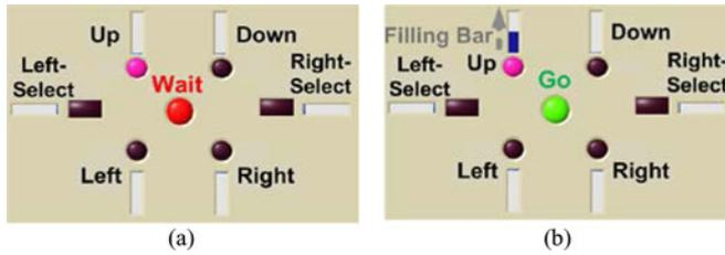
Fig. 4. GUI screen for timed randomly selected commands task from which the TDS ITR can be derived: (a) indicating the random command and being ready, (b) selecting the tongue command and staying there until the blue bar is filled before returning back to neutral.
